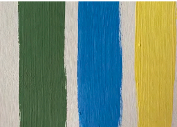
Colour testing showing pigment strengths of eco-paint compared to other brands, showing that eco-paint is fainter
