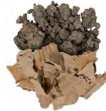
The images above show the three main stages of cellulose fibreboard making process. It starts with paper waste being shredded cellulose fibre, which is then mixed with water binder and fire retardant. Finally the mixture is compressed to form a compact solid board.
